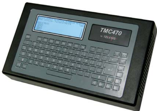
Compact Self-Contained TMC470 Controller — no PC required.
