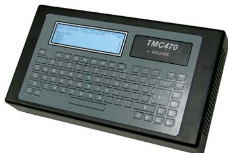
Compact Self-Contained TMC470 Controller — no PC required.
