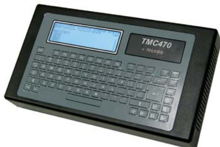
Compact Self-Contained TMC470 Controller — no PC required.
