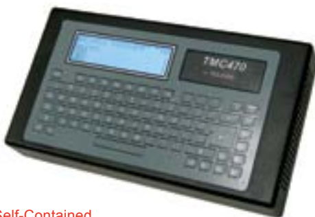
Compact Self-Contained TMC470 Controller — no PC required.
