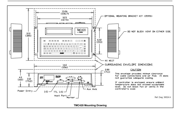
**Environmental Considerations.** The following environmental considerations must be taken into account when installing the TMC420 controller.
